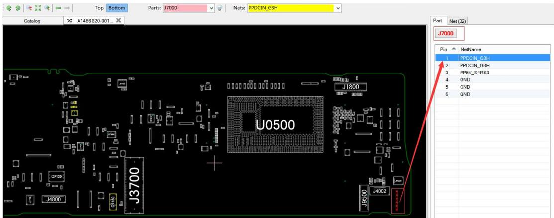
The material object motherboard compares the bitmap, and learns that the name of the battery interface in the circuit diagram is: J7000
