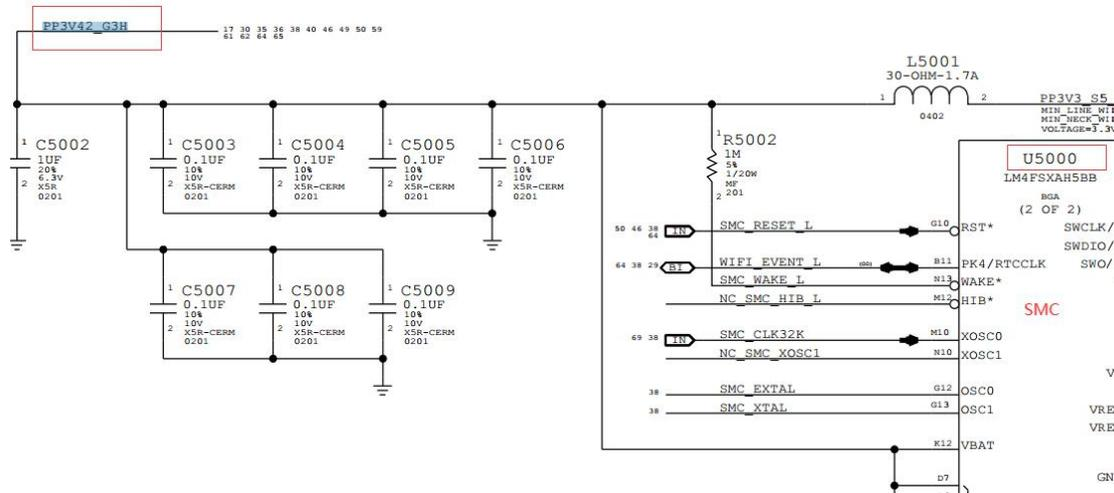
PP3V42\_G3H is the earliest power supply generated on the motherboard (G3 state), at this time the common point voltage has not yet been generated.
