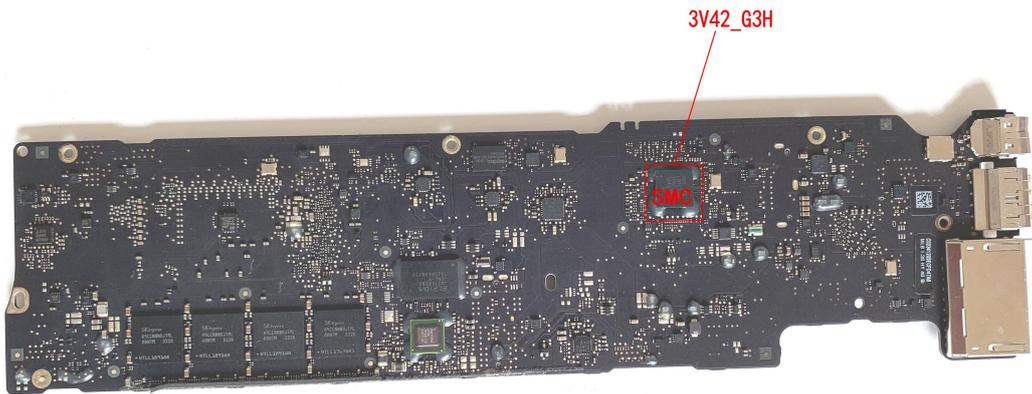
After the SMC works normally, it communicates with the charger through SYS\_ONEWIRE, and the charger lights up in green (the single board turns green to yellow and orange if the battery is not inserted). You can judge whether the SMC is working normally by whether the green light is on.
