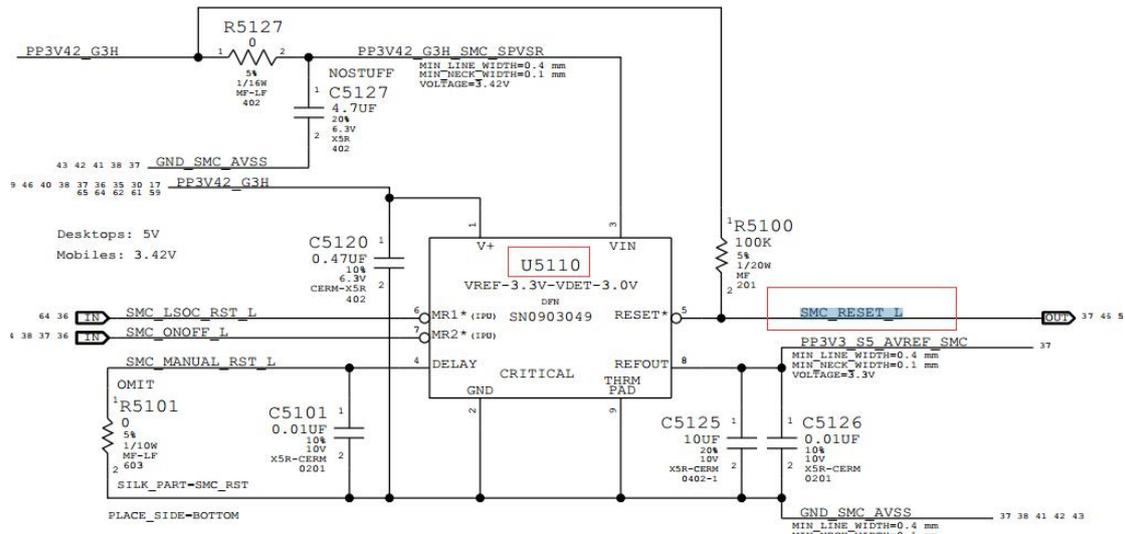
The reset signal voltage output by U5110 is 3.3V
