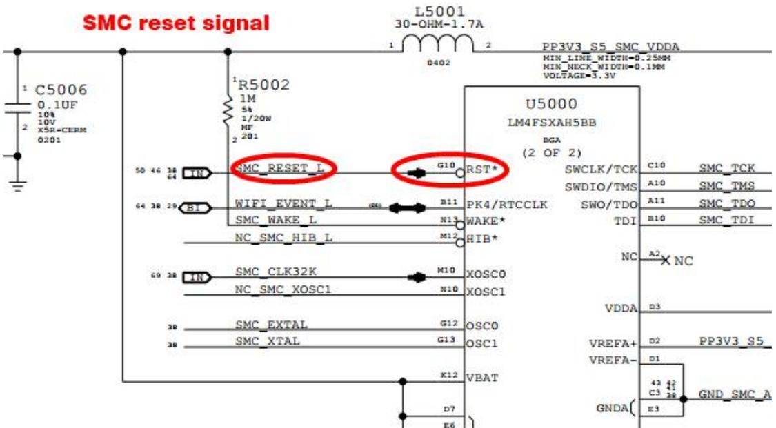
Search for reset signal in the schematic: SMC\_RESET\_L found to come from U5110
