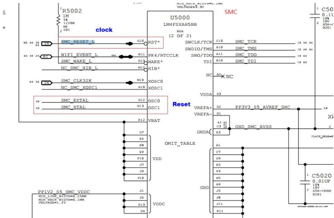
After the SMC satisfies the power supply, reset, and clock, it reads the internal program, starts to configure the pin function, and turns on the South Bridge standby.
