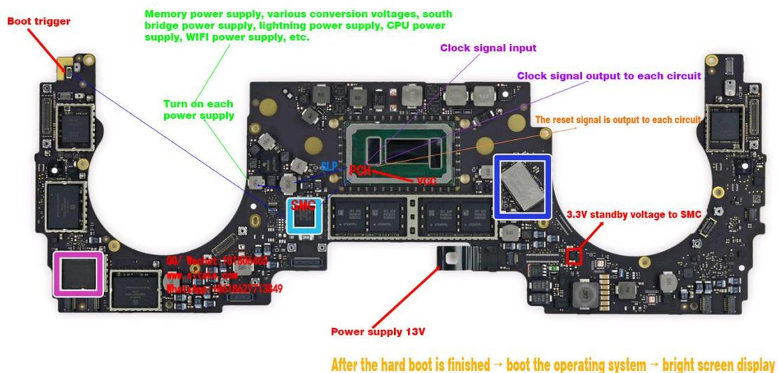
Based on the above, we can divide the power supply of the laptop into 4 levels:
