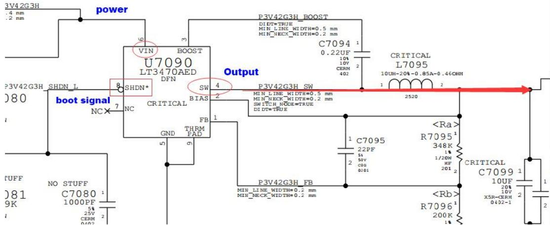
U7090 working conditions are normal, the feedback circuit is also normal, it will output: PP3V42\_G3H, PP3V42\_G3H to supply power to many circuits, but the most important thing is to supply power to the SMC:
