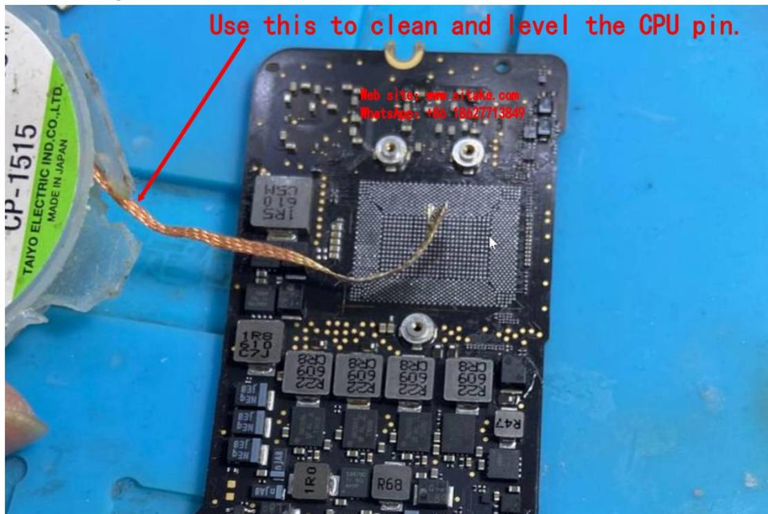
After marking, CPU's pin tin should be cleaned and leveled. Make the mark to make it easy to aim at the position when the chip is put back, just see it clearly, don't push, otherwise the line will be broken.
