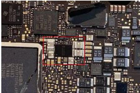
Measure whether the inductor voltage and ground resistance here are normal.
