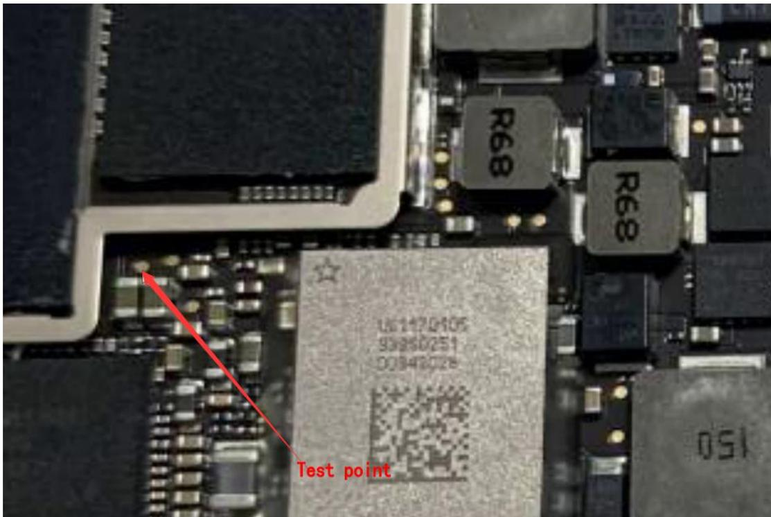
There is a voltage of 1.7v on the test point. When measuring the voltage, it should be noted that if the PCIE bus capacitor is accidentally grounded by the test pen, the CPU will burn. When the voltage is normal, check the reset, turn on, clock signal:
