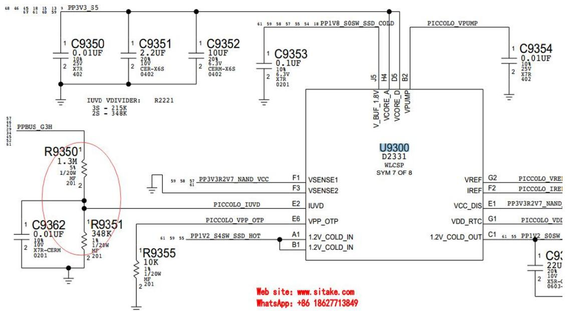
E2 pin 1.7V partial voltage is normal.
